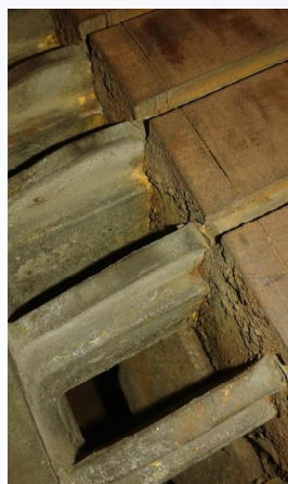
Rotor with visible degradation signs and some broken bars
